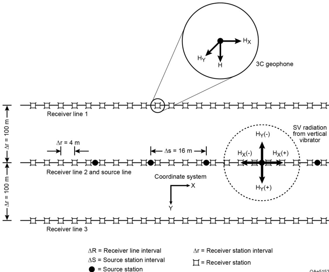
Figure 3. A map view of the type of swath-shooting geometry recommended for 2D profiles across the Zululand Basin.
