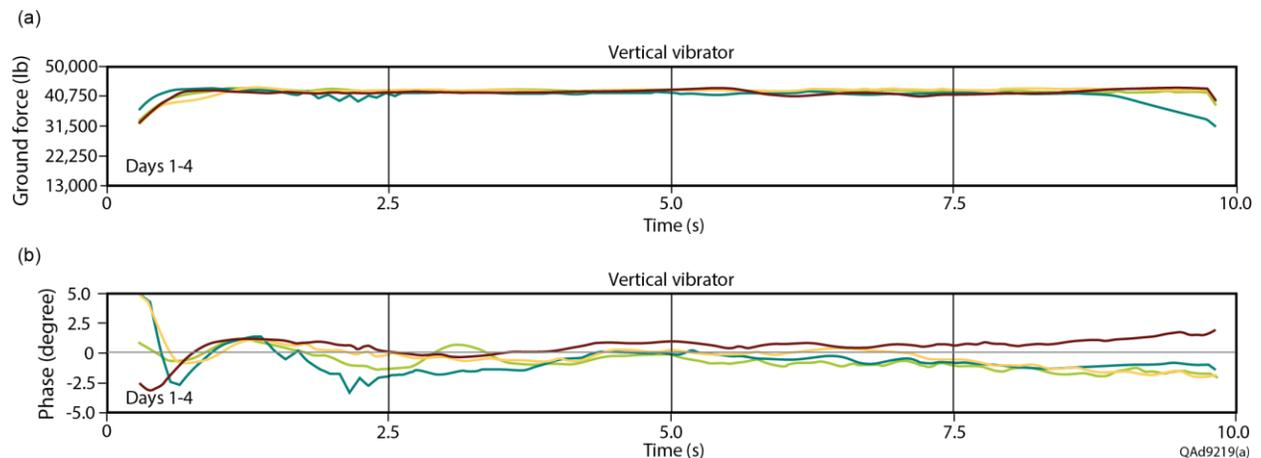
Figure 1. Ground-force phase-lock performance during a seismic data-acquisition program in west Texas. Each display has four curves that represent vibrator performance during 4 successive operating days. (a) Ground force magnitude when a 70-percent drive is utilized during an 8-to-80 Hz, 10-sec sweep. (b) Phase-lock at each of the 73 sweep frequencies stays within 2-degrees of the phase of the corresponding frequencies in the master sweep.
