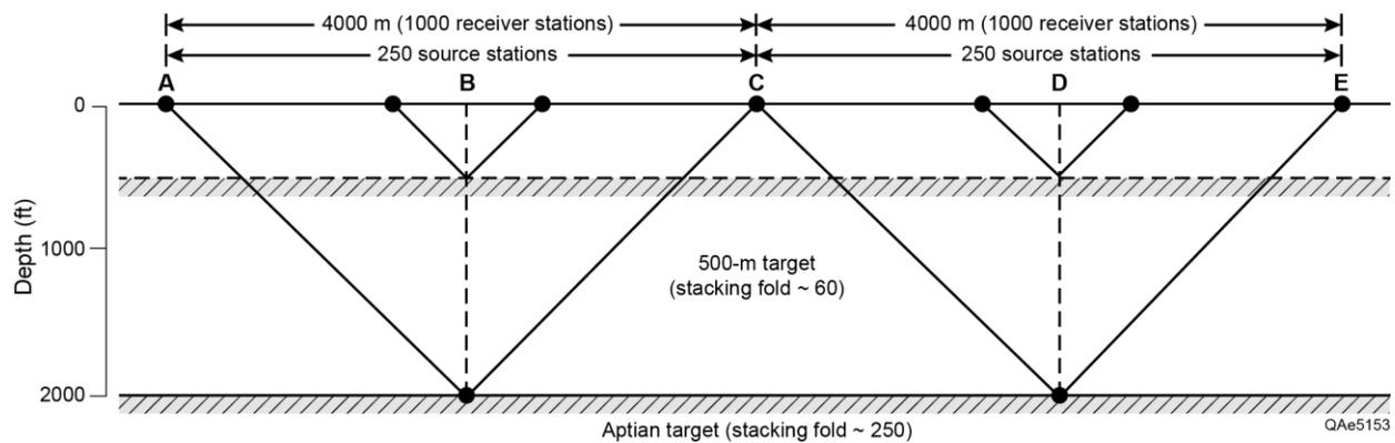
Figure 4. Section view of consecutive receiver spreads appropriate for imaging Aptian sandstones.
