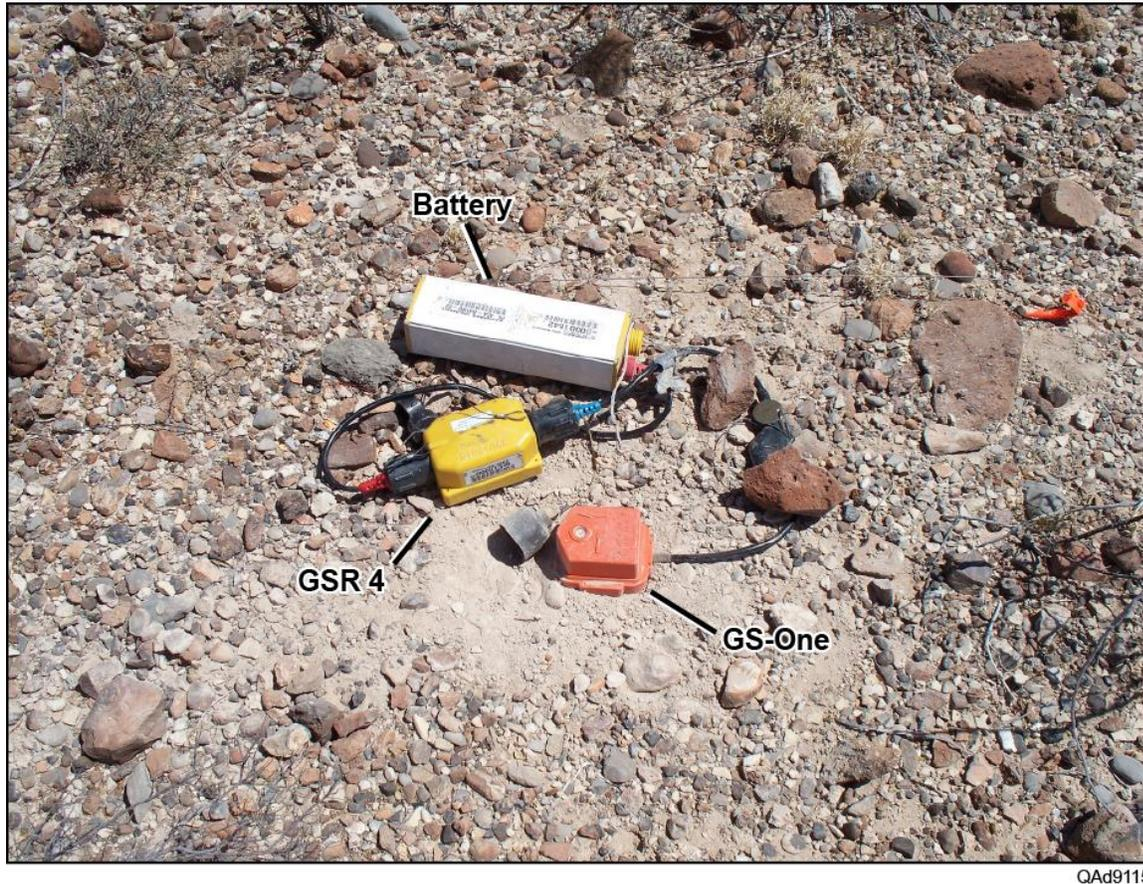
Figure 2. Representative single-point, nodal, receiver station. **GS-One** is a 3C geophone, and **GSR 4** is a 4-channel recorder and electronics package. The **Battery** dimensions are approximately 8-cm (width) and 25-cm (length).
